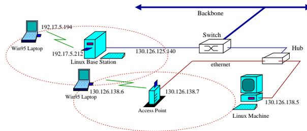
Figure 2: Wireless Testbed
