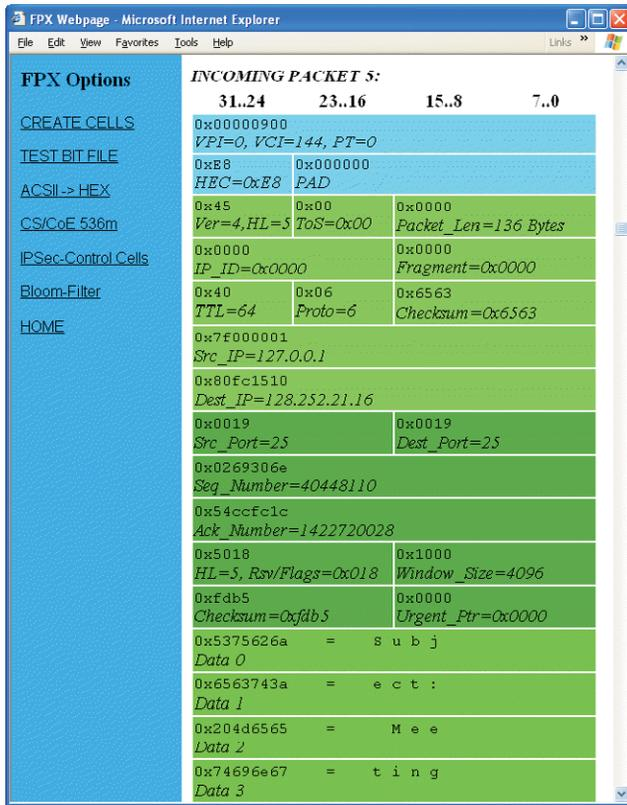
Figure 7: View of packets displayed on test server
