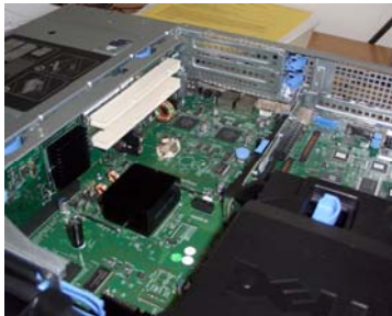
NetFPGA properly recognized in PCI-X slot
