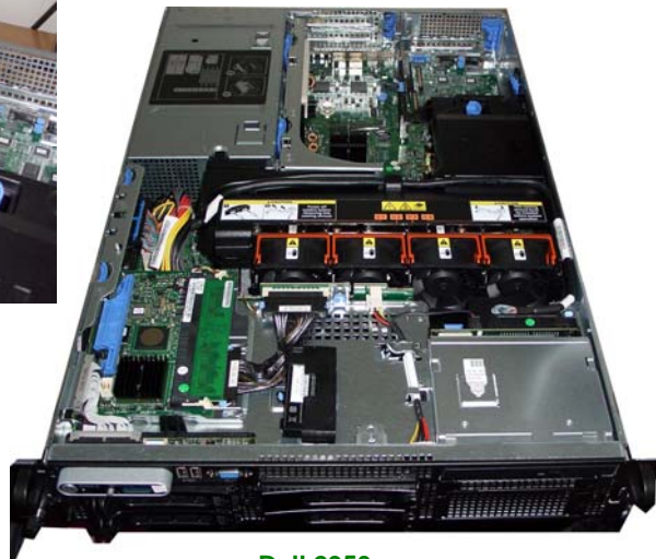
Dell 2950 with PCI-X and PCI-Express Slots
