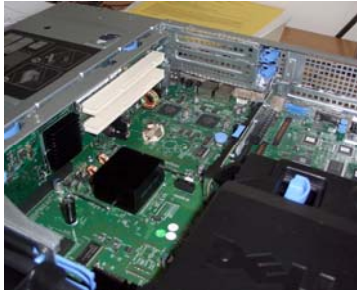
NetFPGA properly recognized in PCI-X slot
