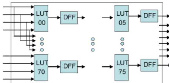
**Figure 2: Basic Structure of Thermal Benchmark Circuits**
