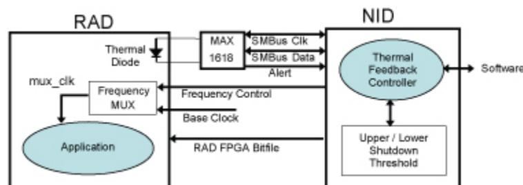
**Figure 3: Modules on the FPX for Thermally Adaptive Computing**
