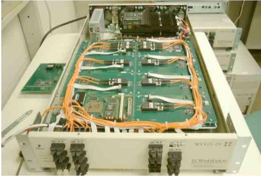
Figure 2: Photo of FPX mounted in WUGS Switch
