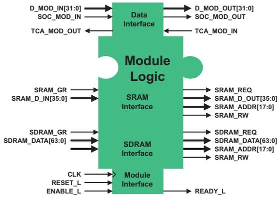
Figure 7: Modular Component of FPX
