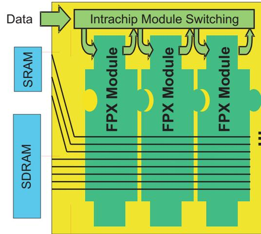
Figure 8: Larger Configuration of FPX Modules
